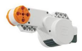
common Lego motors. They are interactive, meaning that they include a built-in Rotation Sensor or tachometer. This lets you control your robot's movements precisely.
