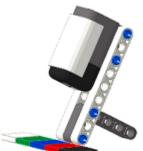
The Colour Sensor connects to an NXT sensor port using a standard NXT wire and digital I2C communications protocol. The *Colour Number* calculated by the sensor is refreshed approximately 100 times per second. It can detect an extended range of more than 15 target colours and the NXT robot can be programmed to react to each colour.
