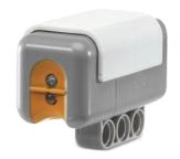
between surfaces of different colors. The NXT generates the light sensor's readings as a percentage. The highest possible reading is 100 percent, which you can easily achieve by holding the sensor up to a light bulb. The lowest possible reading is 0 percent, which you could achieve in a very dark closet.
